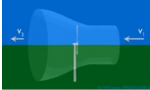
Fig. 3. Wind speed before the wind turbine ( v_1 ) and after the passage through the rotor plane ( v_2 )
